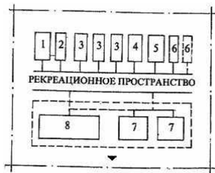
Rice. 4. Functional and planning diagram of a group of administrative and utility rooms
