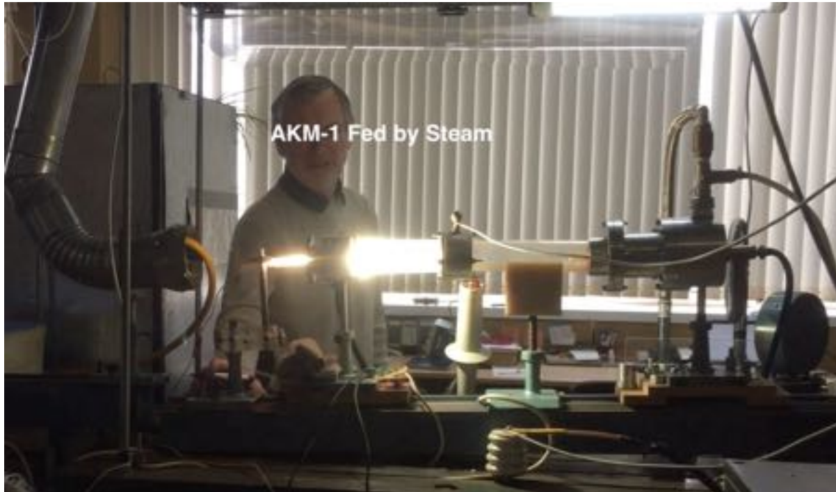
Fig. 5. The plasma in the reactor increased the light emission when the feed was switched to steam. You see the steam fog in the glass tube before the reactor.
